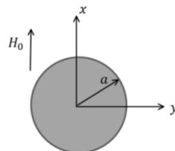
cutting meniscus to the right of the cylindrical magnet with a radius  $a >> D$ . The magnetic field is  $H_0$ .
